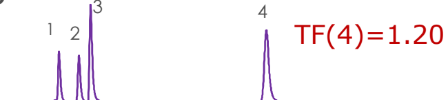
D Brand D C18, 2.6 \mu m core shell type
