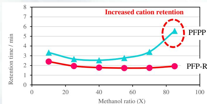
Fig. U-Shape: transition from reversed-phase to normal-phase
