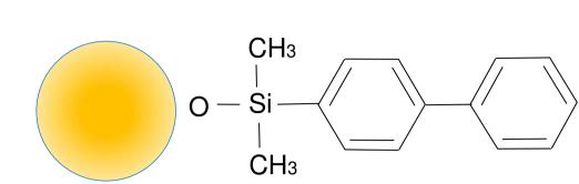
Feature of end-capping of SunShell Biphenyl (sunniest end-capping)
