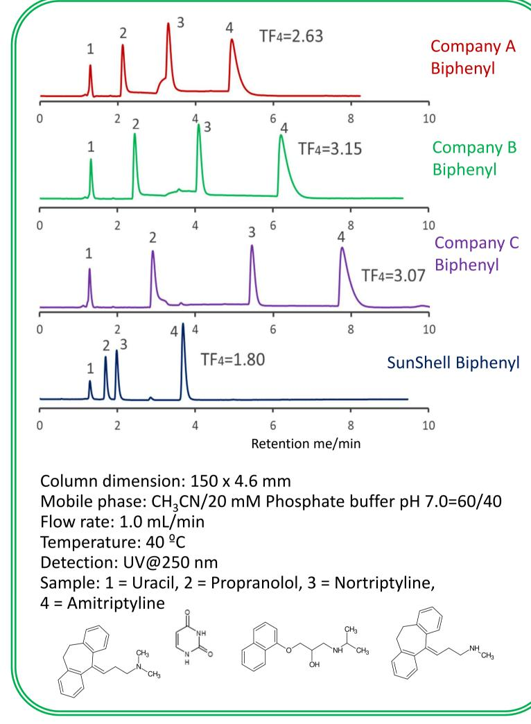
Tailing of basic compounds (amitriptyline) occurs more easily in the acetonitrile/buffer mobile phase than in the methanol/buffer mobile phase. A mixture of acetonitrile and 20 mM phosphate buffer was used as mobile phase to compare with core shell Biphenyls. Biphenyl from other companies had a terrible tailing for basic compounds.
