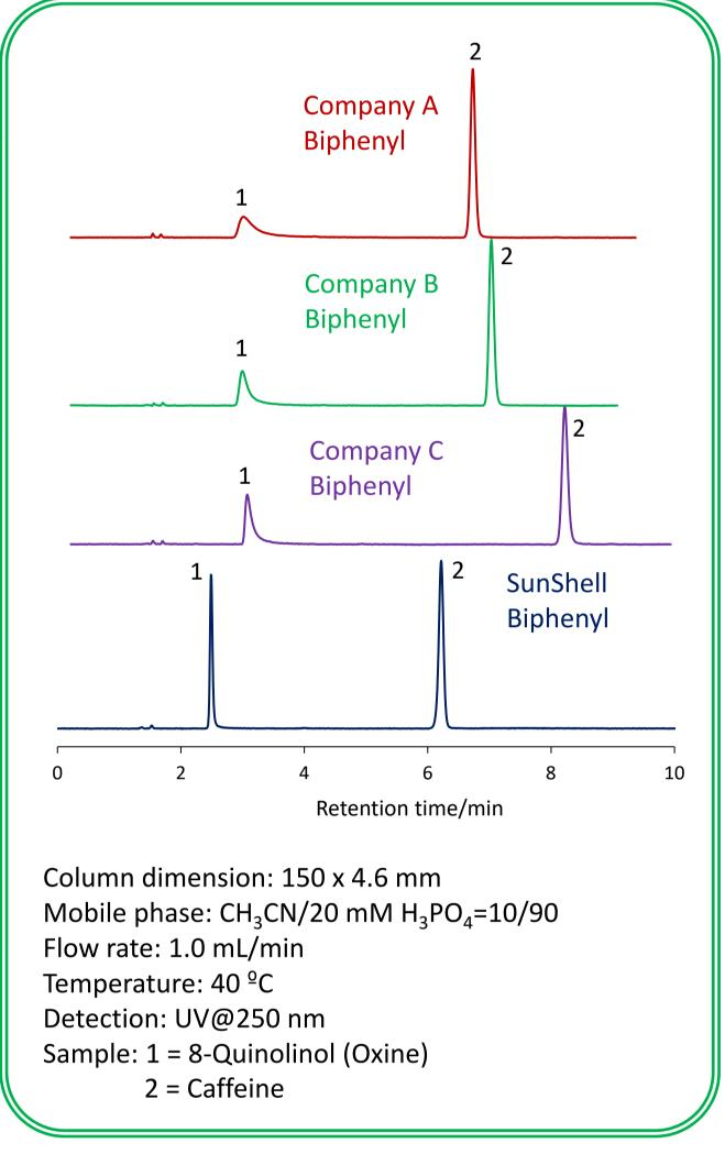
8-Quinolinol (oxine) is a metal chelating compound, and if there are metal impurities in the packing material, its peak becomes a tailing peak.
