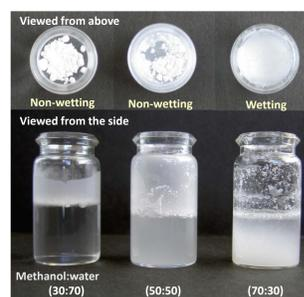
C18 packing materials were put into each solvent and stirred with ultra sonic vibration.
