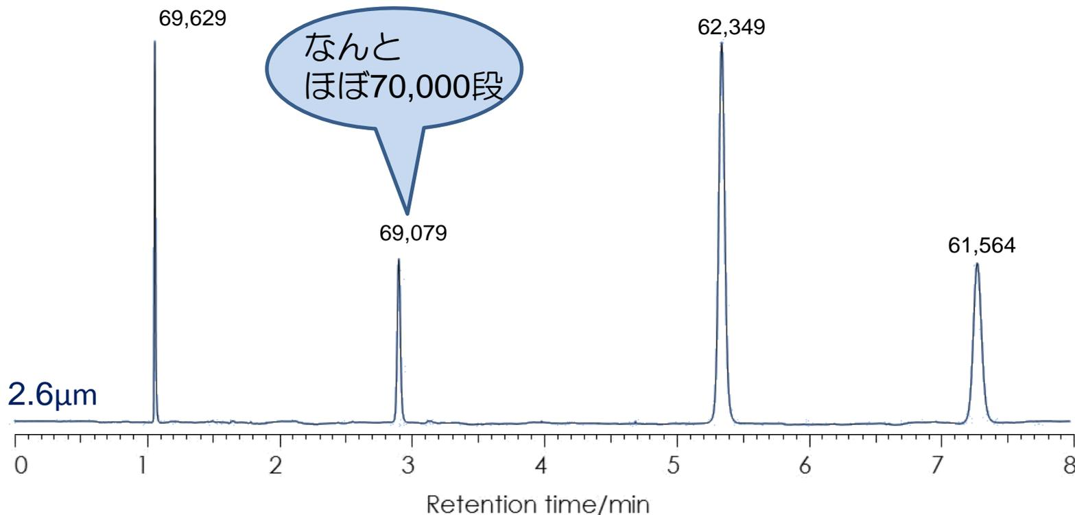
Column: SunShell C18, 2.6 μm, 250 x 4.6 mm
