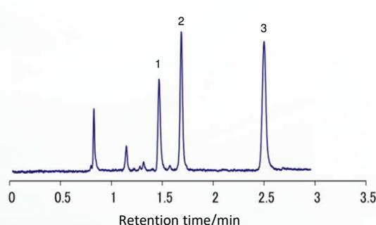
Column: SunShell HILIC-Amide, 2.6  $\mu\text{m}$  100 x 4.6 mm
