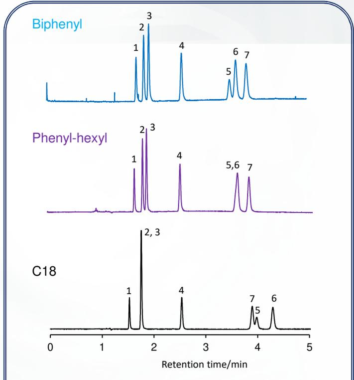
Column: SunShell Biphenyl, Phenyl and C18 2.6  $\mu$ m, 150 x 4.6 mm
