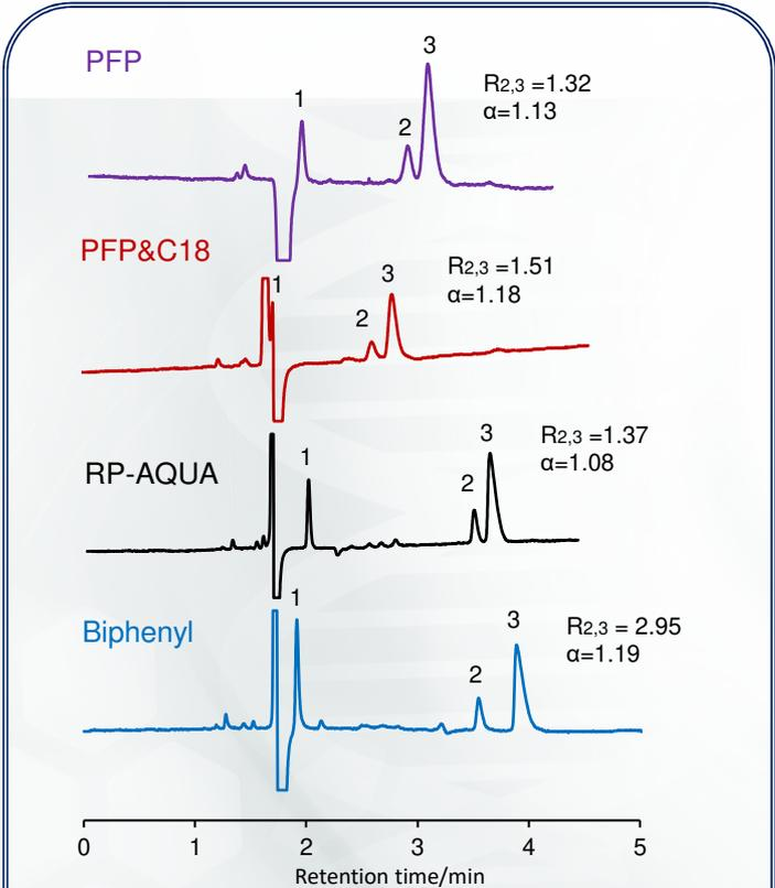
Column: SunShell PFP, PFP&C18, RP-AQUA, Biphenyl 2.6  $\mu$ m, 150 x 4.6 mm
