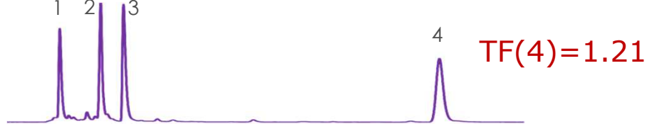
C SunShell C18(HMODTS), 2.6 \mu\text{m} core shell type
