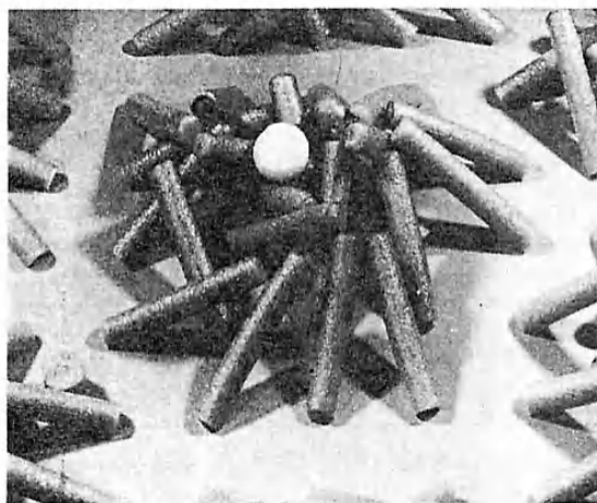
Figure 2. A scaled representation of octadecyl chains chemically bonded to the surface of silica gel showing solvophobic aggregation of the bonded ligands. Appropriate coverage data for this phase was taken from Table II. The white circle on the cluster represents a benzene sized solute molecule.
