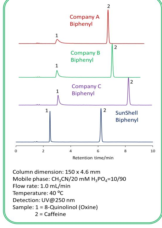
8-Quinolinol (oxine) is a metal chelating compound, and if there are metal impurities in the packing material, its peak becomes a tailing peak.
