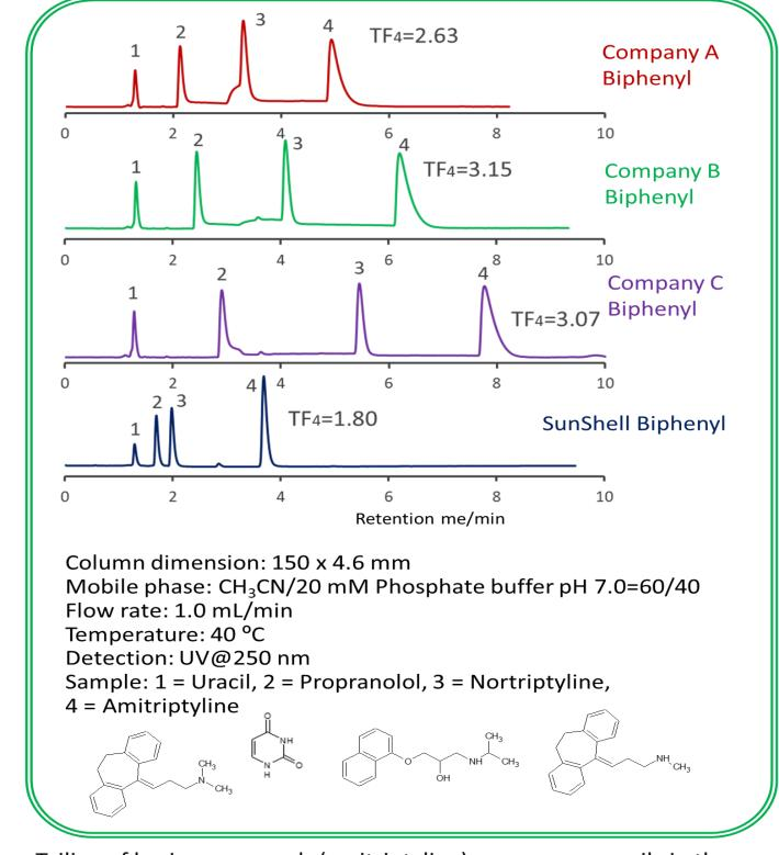
Tailing of basic compounds (amitriptyline) occurs more easily in the acetonitrile/buffer mobile phase than in the methanol/buffer mobile phase. A mixture of acetonitrile and 20 mM phosphate buffer was used as mobile phase to compare with core shell Biphenyls. Biphenyl from other companies had a terrible tailing for basic compounds.
