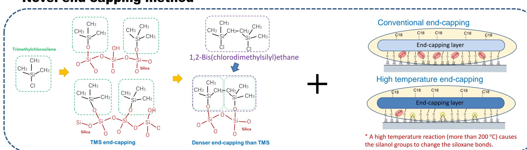
ArmorShell C18: 2.6 µm of core shell silica bonded with trifunctional C18 and end-capped using the above novel end-capping method. C18 of Company A and Company B uses hybrid core-shell silica in which ethylene chains are bonded on the silica surface. (Kinetex EVO C18 and PoroShell HPH C18)
