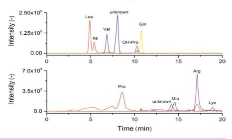
LC–MS System: Agilent 1100er LC system and Thermo Fisher LTQ<sup>TM</sup> equipped with a HESI source, operated in positive ionization mode for analysis of standards. For the dietary supplement, an Orbitrap<sup>TM</sup> Exactive classic equipped with a HESI source and operated in positive ionization mode. Column: iHILIC-Fusion(+)  $3.5 \,\mu m$   $100 \mathring{\text{A}}$ ,  $150 \times 2.1 \,mm$  i.d.
